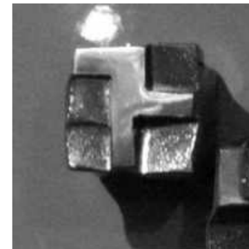
iron blocks deformed by external force size about 40x40mm
